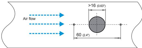
The arrow engraved on the sensing head of EE660 indicates the direction of the air stream during factory adjustment. When installing the EE660 probe, make sure that the arrow matches exactly the flow direction.
