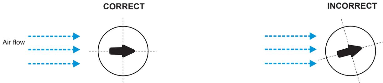
The mounting flange allows for precise setting of the EE660 immersion depth in a duct. The entire sensing head must be in the air flow to be measured.
