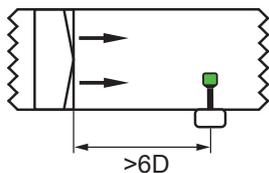
The preferred position of the sensor is after a filter.
