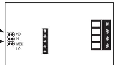
For performing EE660 settings via EE-PCS Product Configuration Software (download from [www.epluse.com/configurator](http://www.epluse.com/configurator)) the working range jumper must be on HI.
