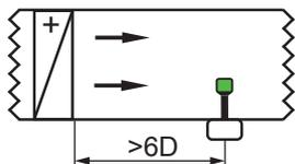
Place the sensor at a position with laminar (non turbulent) flow. Turbulence appears after fans as well as after bends, junctions, air heater, air cooler, filters, flaps or diameter changes in the duct.
