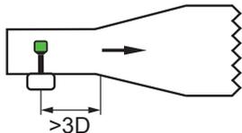
Place the sensor in front of the diffusers at a position with high air velocity.
